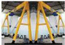
Single Girder Gantry Crane (5 Ton)
