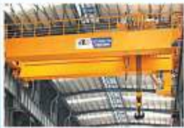
Double Girder Crane (25 Ton)
